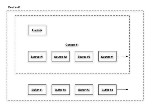
When initializing OpenAL, at least one device has to be opened. Within that device, at least one context will be created. Within that context, one listener object is implied, and a multitude of source objects can be created. Each source can have one or more buffers objects attached to it. Buffer objects are not part of a specific context – they are shared among all contexts on one device.
