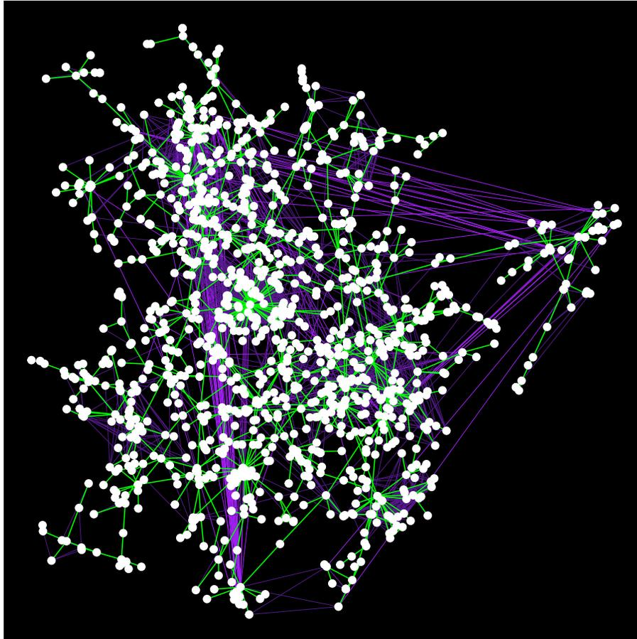
**Figure 12:** Global layout style of the *A. Thaliana* network. The position of the nodes in the MST are determined by Fruchterman-Reingold, edges found by the MST are shown in green, other edges are shades of purple.
