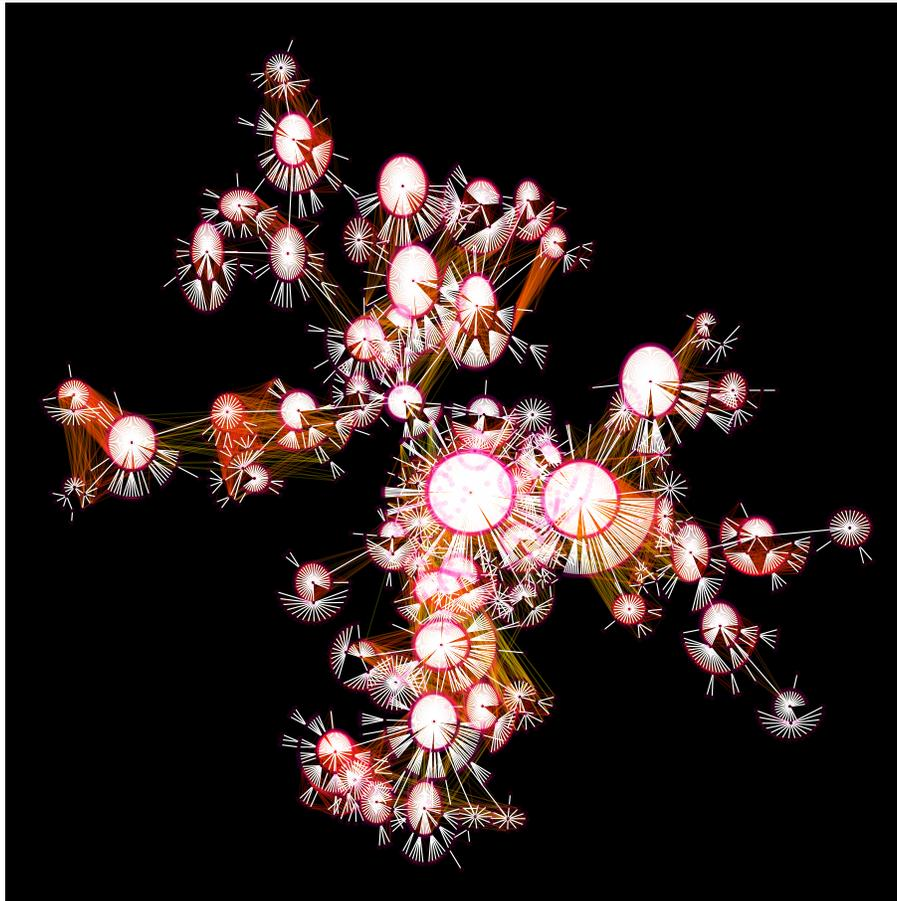
**Figure 2:** Global layout style of artificial network 2 ( $|V| = 5,000$ ,  $|E| = 23,878$ ). Position of the nodes in the MST are determined by combining the Reingold-Tilford and the Kamada-Kawai algorithm. Edges found by the MST are white, other edges are shades of red to yellow.
