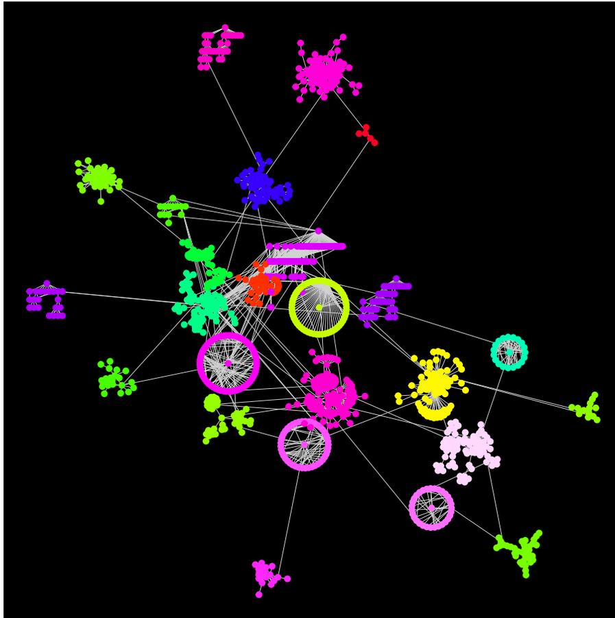
**Figure 18:** Modular layout style of the *A. Thaliana* network. The position of different modules is determined by different layouts given as inputs to the function. Colors for the modules are chosen randomly from a compiled list of bright colors.
